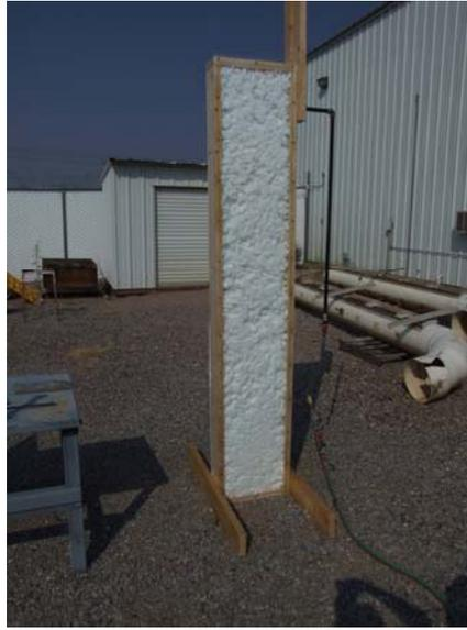
**Figure 17 – View showing the plexiglass-covered side of the full-scale fire model prior to testing.**
