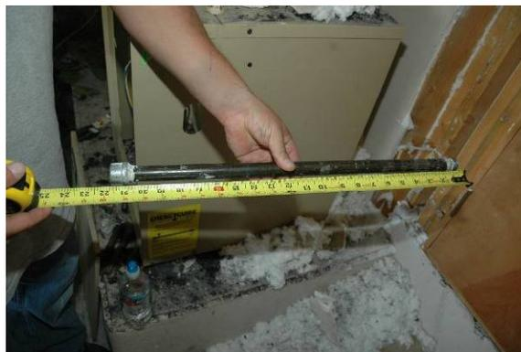
**Figure 8 – The 21-inch long section of gas pipe which was removed from the wall cavity by the workman on the day of the fire.**
