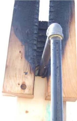
**Figure 21 – The fire pattern created at the top of the full-scale fire model after the burn testing.**
