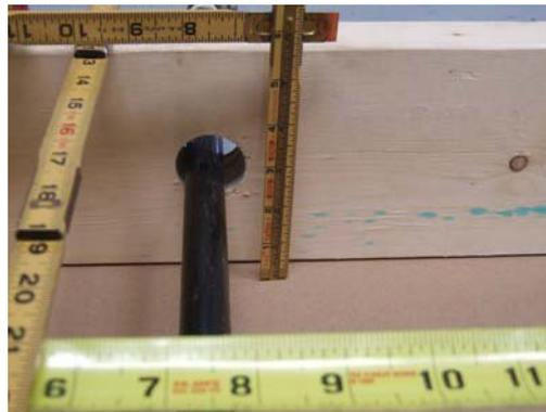
**Figure 15 – The enlarged hole where the gas line entered the full-scale fire model wall cavity.**
