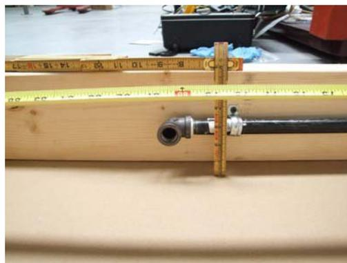
**Figure 16 – The elbow near the bottom of the full-scale fire model where the gas escaped when the 21-inch pipe was unscrewed.**
