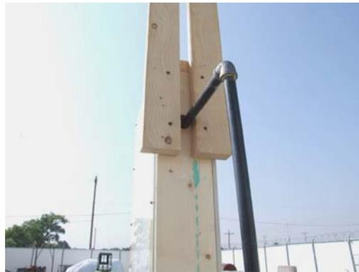
**Figure 18 – The location near the top of the full-scale wall cavity where the gas line entered the cavity.**
