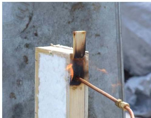
**Figure 13 – The one-quarter scale fire model during testing.**
